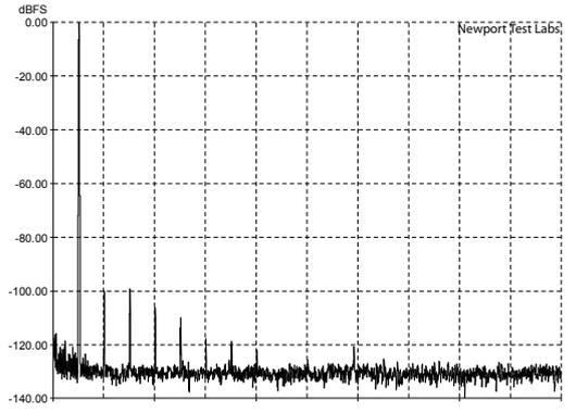
Graph 2: Total harmonic distortion (THD) at 1kHz at an output of 1-watt into a 4-ohm non-inductive load, referenced to 0dB. [Cambridge Audio Azur 851E & 851W Pre/Power Amps]
