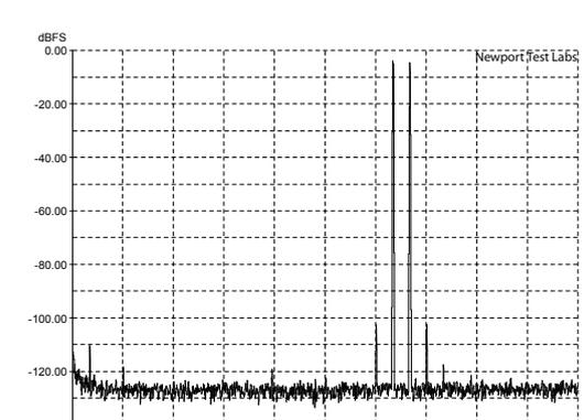
Graph 8: Intermodulation distortion (CCIF-IMD) using test signals at 19kHz and 20kHz at an output of 1-watt into an 8-ohm non-inductive load, referenced to 0dB. [Camb. 851E/851W]
