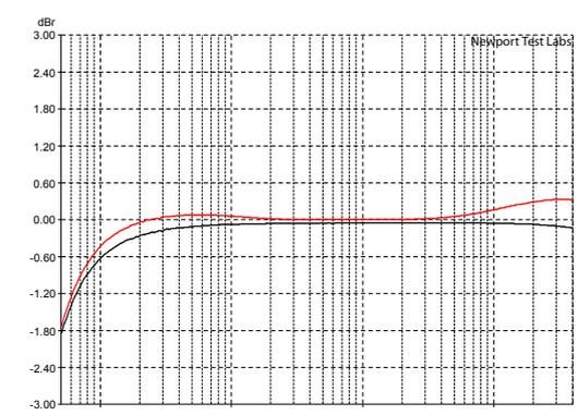
Graph 6: Frequency response of line input at an output of 1-watt into an 8-ohm non-inductive load with 'Direct' mode (black trace) engaged, and with tone controls in 0dB position (red trace). [Cambridge Audio Azur 851E & 851W Pre/Power Amplifiers]
