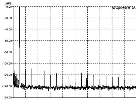
Graph 3: Total harmonic distortion (THD) at 1kHz at rated output (200 watts) into an 8-ohm non-inductive load, referenced to 0dB. [Cambridge Audio Azur 851E & 851W Pre/Power]
