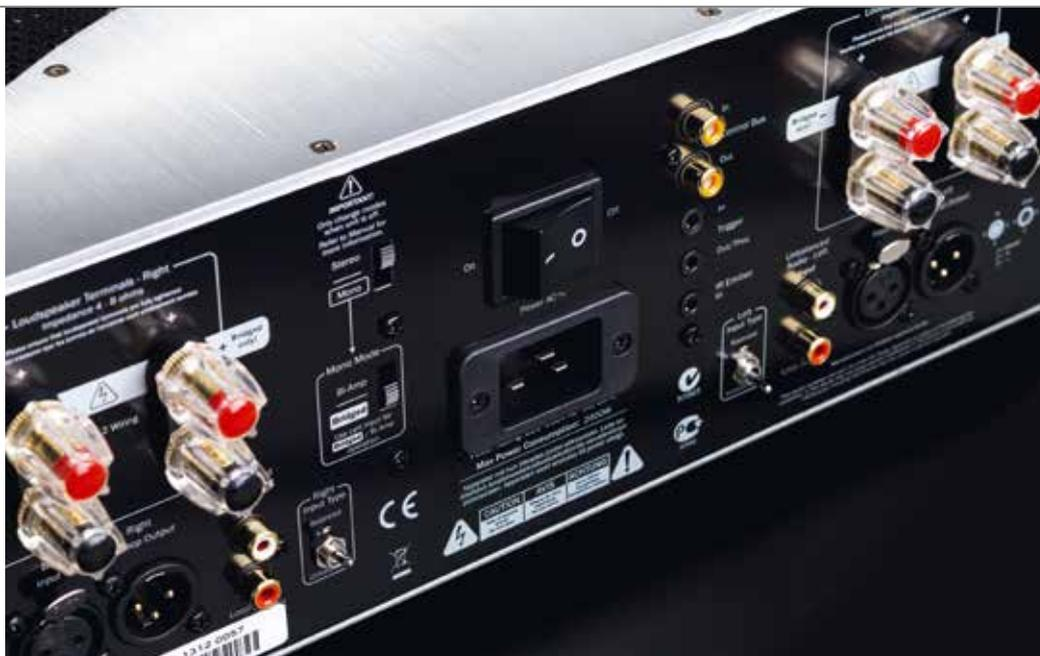
bi-amplified 'monobloc' amplifier, in which case 'Mono' would glow, or as a dedicated mono amplifier, with the outputs of the left and right channels bridged into just a single channel, in which case the 'Bridged' LED would glow and you will benefit from a substantial increase in output power (up from 200 watts to 500-watts according to Cambridge Audio's specifications, but rather more according to bench testing conducted by *Newport Test Labs*).
