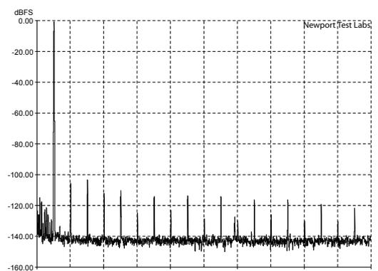
Graph 4: Total harmonic distortion (THD) at 1kHz at rated output (350 watts) into a 4-ohm non-inductive load, referenced to 0dB. [Cambridge Audio Azur 851E & 851W Pre/Power]
