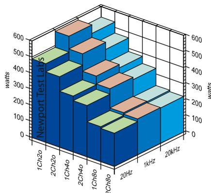
Power Output: Single and both channels driven into 8-ohm, 4-ohm and 2-ohm non-inductive loads at 20Hz, 1kHz and 20kHz. [CA 851W]
