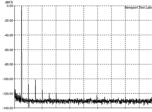
Graph 1: Total harmonic distortion (THD) at 1kHz at an output of 1-watt into an 8-ohm non-inductive load, referenced to 0dB. [Cambridge Audio Azur 851E & 851W Pre/Power]
