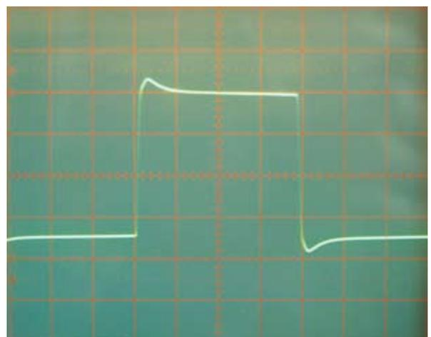
1kHz Square Wave (8Ω//2uF capacitive load)
