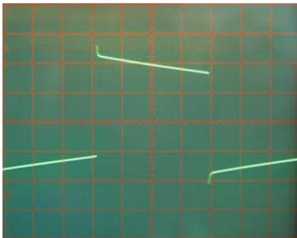
100Hz Square Wave (8Ω resistive load)
