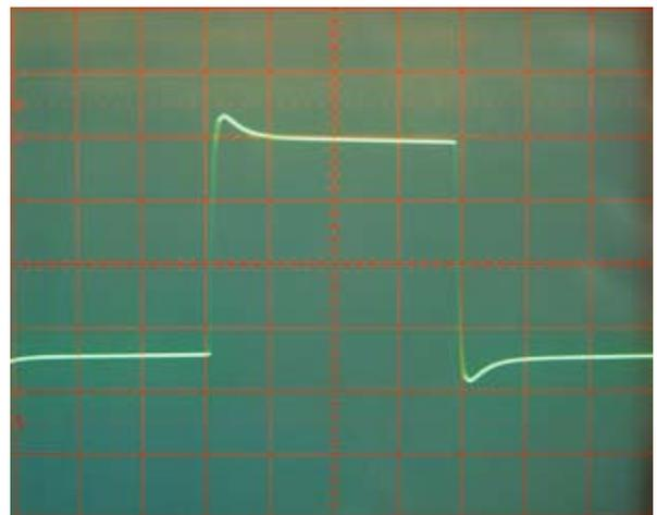
1kHz Square Wave (8Ω resistive load)
