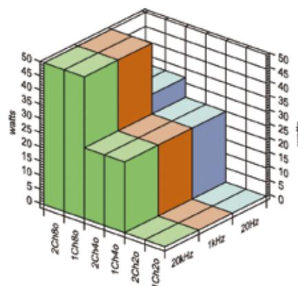
Power Output: Single and both channels driven into both 8Ω and 4Ω loads, in both instances using the 8Ω tap on the Kronzilla's output transformer.
