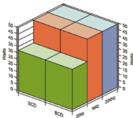
Power Output: Single and both channels driven into 8Ω non-inductive loads.
