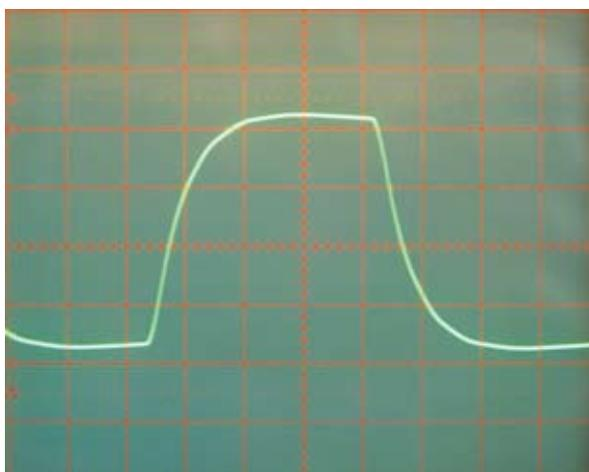
10kHz Square Wave (8Ω resistive load)
