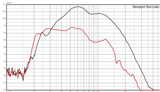
Figure 4: Nearfield sine frequency response of bass driver (black trace) and down-firing passive radiator (red trace) when using high-level inputs with crossover set to 40Hz. (Note that data for has not been re-scaled to compensate for differences in radiating areas.) [GoldenEar ForceField 4]
