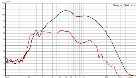
Figure 3: Nearfield sine frequency response of bass driver (black trace) and down-firing passive radiator (red trace) when using LFE input. (Note that data for has not been re-scaled to compensate for differences in radiating areas.) [GoldenEar ForceField 4 Subwoofer]
