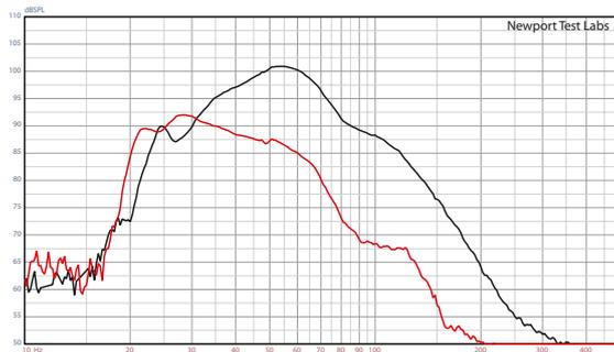
Figure 5: Nearfield sine frequency response of bass driver (black trace) and down-firing passive radiator (red trace) when using high-level inputs with crossover set to 150Hz. (Note that data for has not been re-scaled to compensate for differences in radiating areas.) [GoldenEar ForceField 4]
