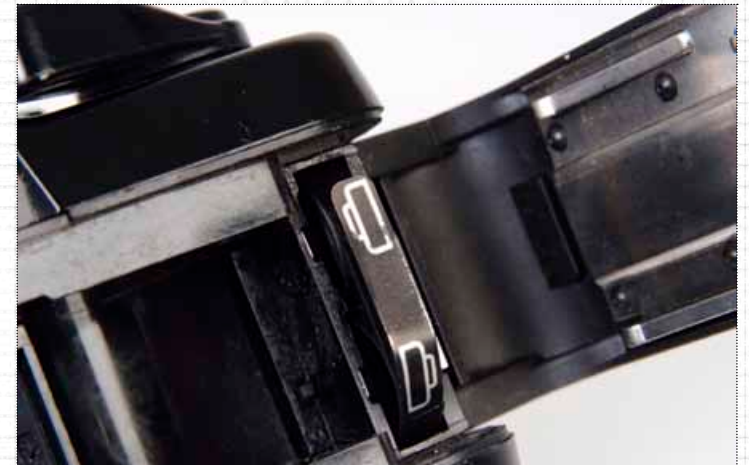
✦ A pair of button cells power the camera and fit into a holder which is then located inside the film cartridge chamber.
