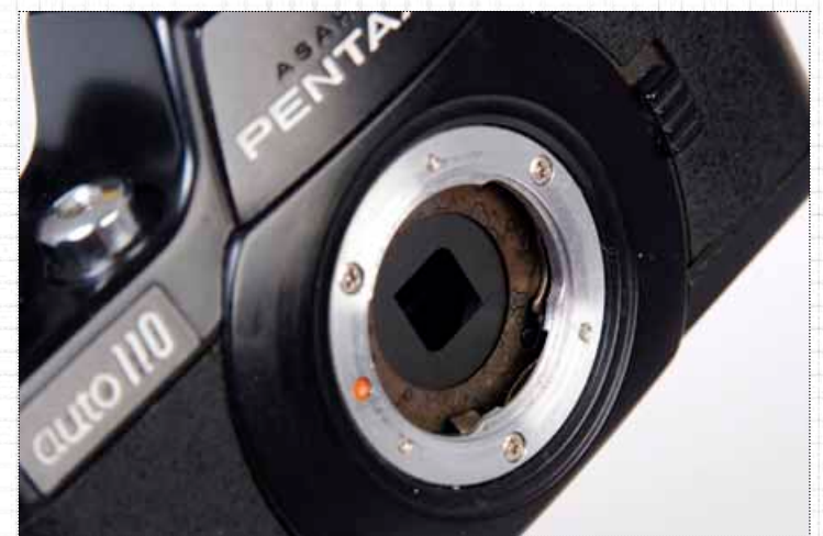
✦ One of the clever design features of the Auto 110 is its combined shutter/diaphragm mechanism located just inside the lens mount on the camera body.
