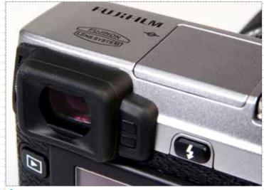
The X-Pro1's hybrid optical/electronic viewfinder is replaced with a purely electronic display, but it's an excellent OLED type with a resolution of 2.36 megapixels. Eyepiece now has strength adjustment built in.
