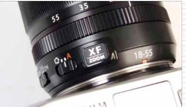
➡ Switch on the 18-55mm zoom's barrel sets the aperture control collar for manual operation or the 'A' for auto aperture control.
