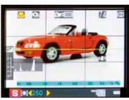
The 'Custom' live view display can be configured to include a wide selection of indicators plus a level display, a realtime histogram, a choice of grids and a distance scale
