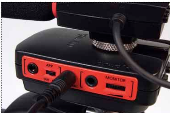
✦ The SmartLynk has an audio output for connecting headphones and (at the far left of this image) an output to an iPhone or iPod also for monitoring purposes via the My Myk Camera Audio app.
