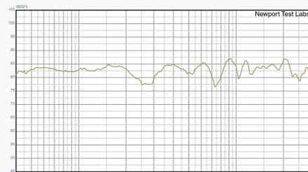
Graph 2. High-frequency response, expanded view. Test stimulus gated sine. Microphone at three metres on-axis with dome super tweeter. Lower measurement limit 400Hz. [JBL LS80 Loudspeaker]
