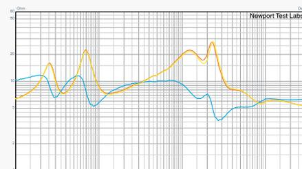
Graph 4. Impedance modulus of left (red trace) and right (yellow trace) speakers plus phase (blue trace). [JBL LS80 Loudspeaker]
