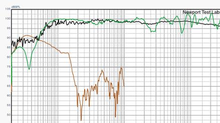
Graph 5. Frequency response. Composite plot. Black trace shows unsmoothed pink noise response (from Graph 1). Green trace is the summed nearfield sine response of the bass drivers spliced (at 400Hz) to the far-field gated response of the tweeter and super-tweeter. The red trace is the nearfield response of the bass reflex port. [JBL LS80 Loudspeaker]
