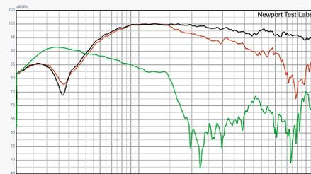
Graph 3. Low frequency response of both woofers and rear-firing bass reflex port (green trace). Nearfield acquisition. Upper woofer (Black). Lower woofer (Red). Port/woofer levels not compensated for differences in radiating areas. [JBL LS80 Loudspeaker]
