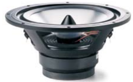
The basket is an enormously heavy casting that has only four narrow support struts, so that no air can be trapped between the rear of the cone and the frame.
