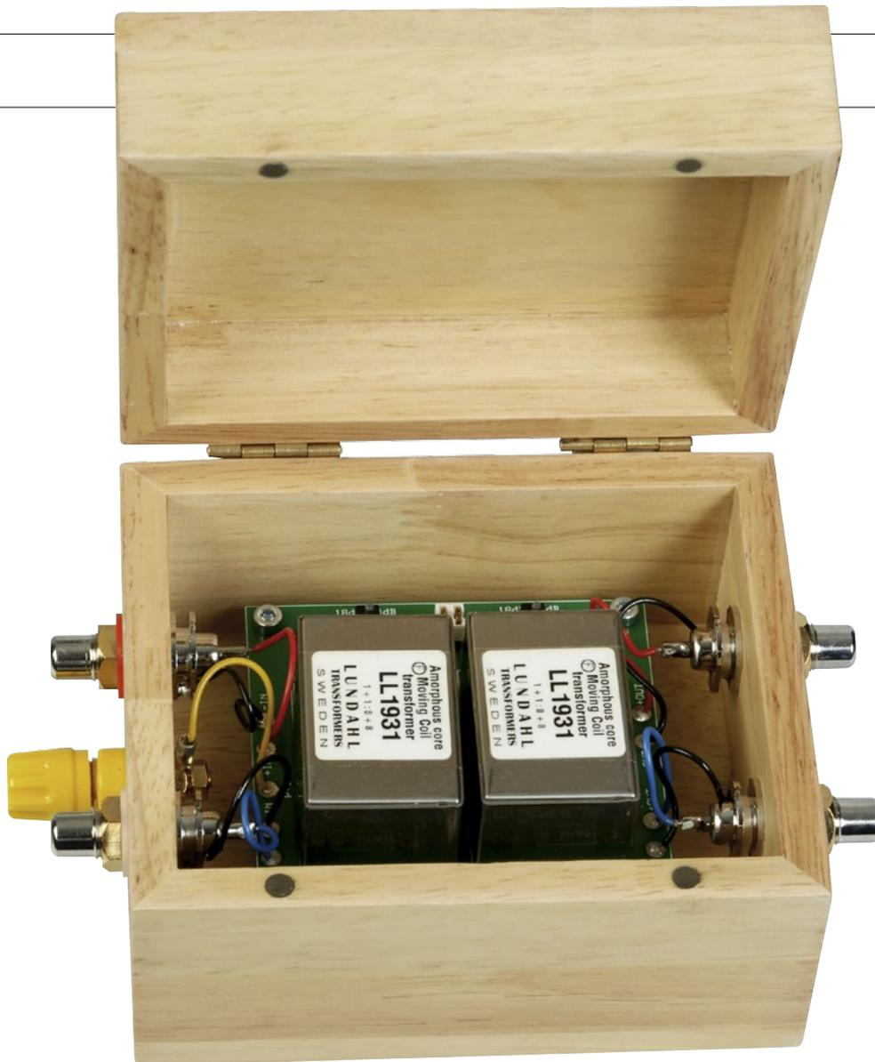
mu-metal transformer,' he said. 'The brush strokes are broader with the mu-metal core transformer and they convey more "body", whereas the amorphous core transformer offers finer brush strokes, which results in hearing more of the details while listening to the whole.' So it would seem to us that Carter preferred the sound of the amorphous core transformer... which is nice because it's the lower-cost option.
