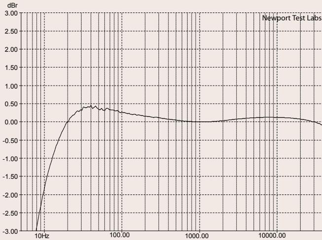
Graph 1. RIAA-corrected frequency response, unbalanced output.
