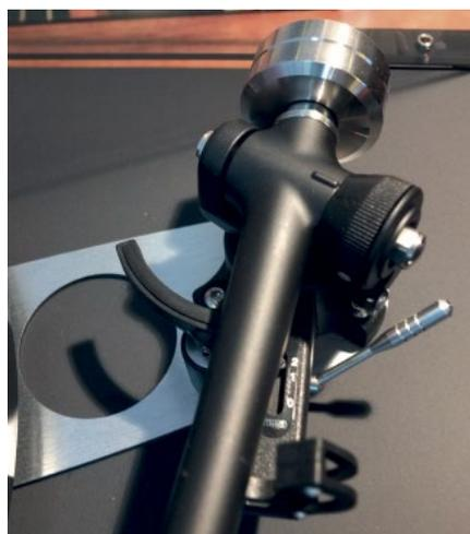
'stressed beam' assembly). It's 'double' because two different materials are used for the stressed beam—not specifically stated here but previously magnesium on top and phenolic resin on the bottom. Combining the two different materials lowers the influence of airborne vibrations on both elements.
