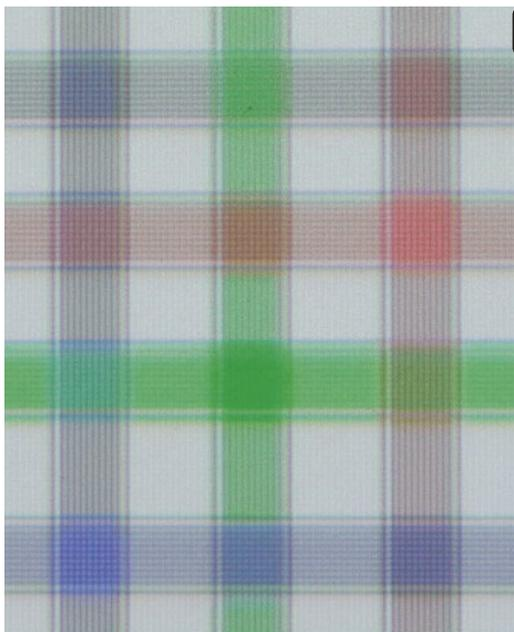
ABOVE: a detail from a photographic image of single-pixel lines in a UHD test pattern (see main copy), as displayed by the BenQ W1700. Note the lines are individually reproduced — not entirely cleanly, and not quite as brightly in colour at the pixel level as when they are reinforced by neighbours, but certainly pixel-for-pixel Ultra High Definition.
