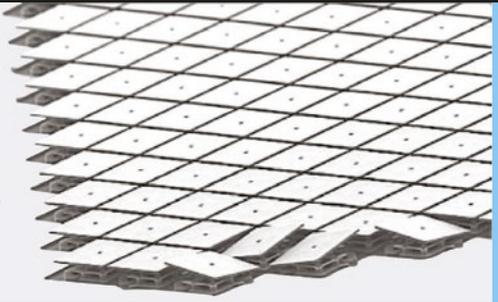
replied that: "The DLP470TE uses a 1920x1080 array of micromirrors, which switch on the order of microseconds, to create four distinct addressable pixels on the screen during every frame to deliver full 4K UHD resolution... The complete set of pixels are oversampled and processed by unique TI image processing algorithms leading to a crisp, colorful & detailed full 8-megapixel 4K UHD display."
