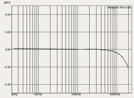
Remember, too, that this is ordinary Red Book CD testing! Inter-channel phase was also outstandingly good, coming in at 0.01° at 20Hz, with a ‘worst’ result of just 0.81° at 20kHz. THD+N was a vanishingly low 0.002% at 1kHz at 0dB and the distortion
