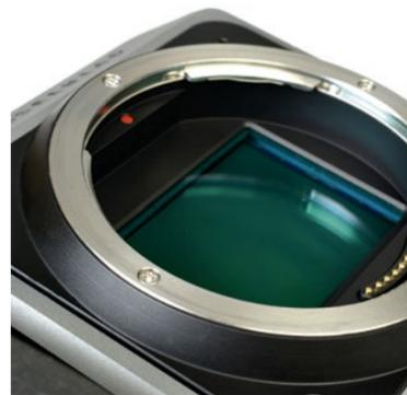
The sensor is another version of Sony's ubiquitous 44x33 mm CMOS imager which has an effective resolution of 51.3 megapixels. Hasselblad has ordered its own design tweaks.
