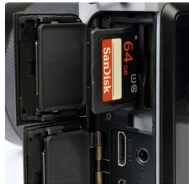
The memory card compartment and connection bay are very neatly integrated into the side of the camera body. Flush-fitting covers slide out to unlock.
