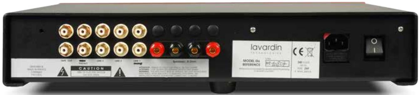
The speaker terminals are not identified as positive or negative, nor are they identified as 'Left' or 'Right'. The RCA inputs are not identified either.
