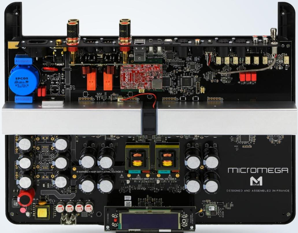
ABOVE: The main circuit board with the ‘cooling tunnel’ clearly visible through the centre. The M-150 differs from the M-100 with the addition of a Power Correction Function and the doubling up of audio amplifier components.
