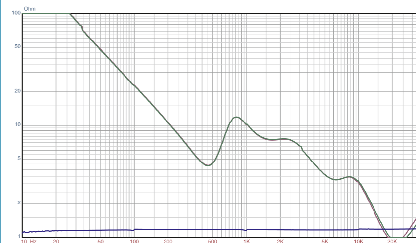
Figure 2: Impedance vs frequency, with both left and right speakers graphed (see copy). Trace under is that of a reference 1Ω precision resistor, measured at the same time for calibration purposes.
